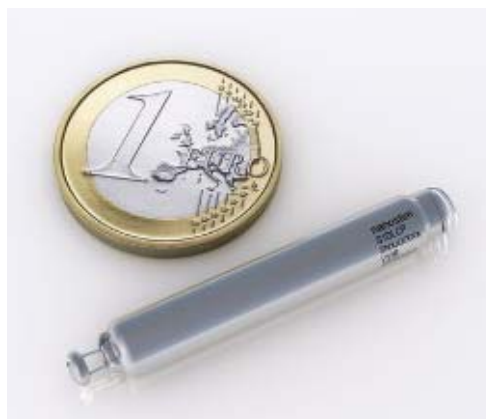
Fig.6. Implanted rate-responsive (intracardiac) pacemaker [31]
