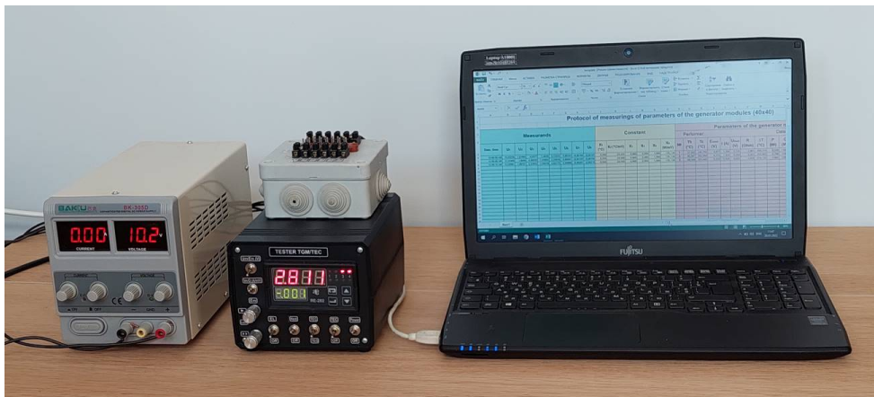
Fig. 2. Appearance of the automation system for measuring parameters of thermoelectric generator modules.
