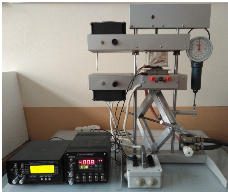
Fig. 1. Appearance of equipment for measuring parameters of thermoelectric modules.
