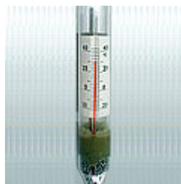
Fig.1. Hydrometer AEF / tosol cooling fluid, antifreeze.
