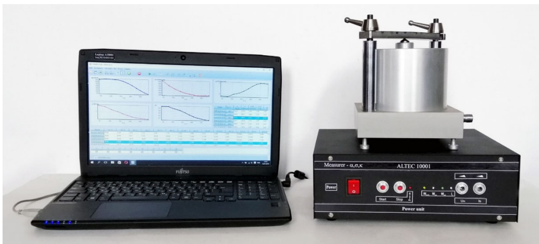
Fig. 1. "ALTEC-10001" installation for measuring the thermoelectric properties of materials by the complex absolute method, developed at the Institute of Thermoelectricity of the National Academy of Sciences and the Ministry of Education and Science of Ukraine.
