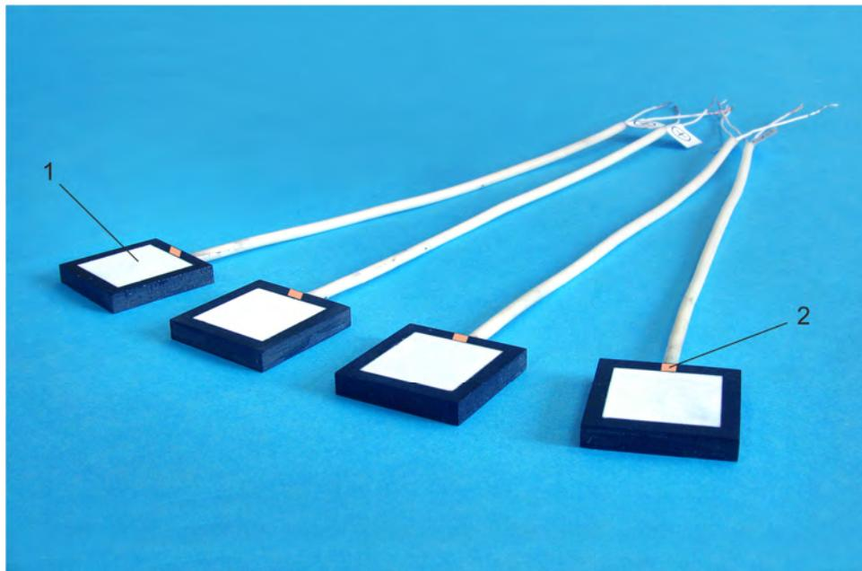
*Fig. 4. Visualization of experimental models of HFS with dimensions of 16×16×3 mm:
