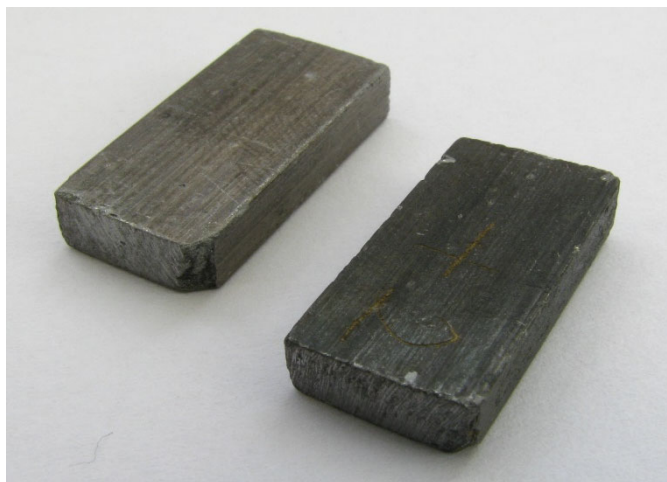
Fig. 1. Extruded bars of thermoelectric material of n- and p-type conductivity.
