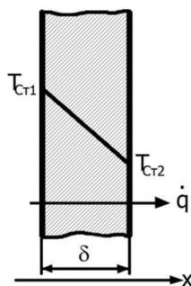
*Fig. 3. Temperature distribution in a flat wall.*
