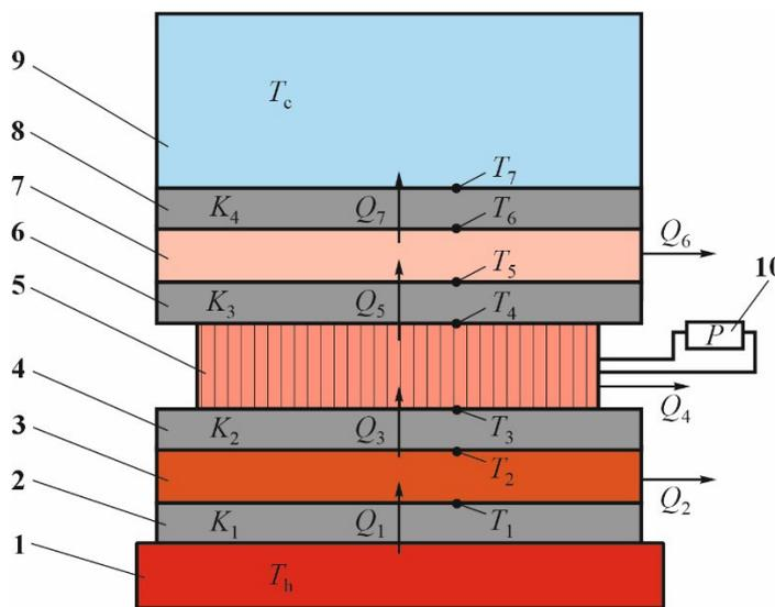
Fig. 2. Physical model of a portable universal thermoelectric generator:
