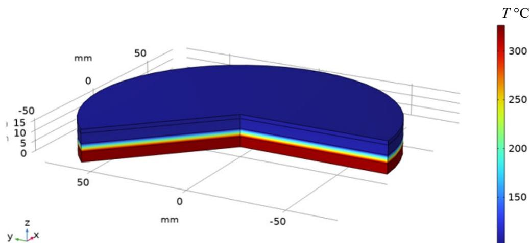
Fig. 7. Temperature distribution in a portable universal thermoelectric generator at time  $t = 3600$  s.
