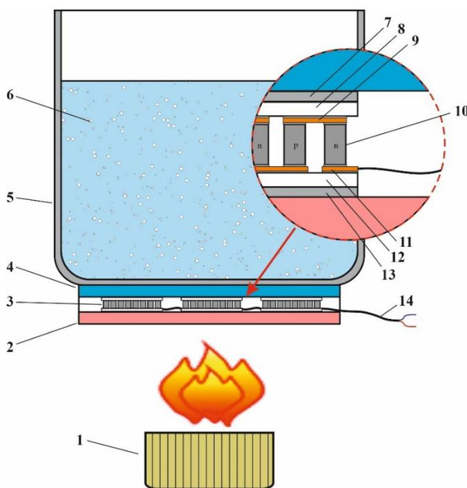
Fig. 1. Design of a portable universal thermoelectric generator: 1 – heat source (heated surface); 2 – “hot” heat exchanger; 3 – thermoelectric generator modules; 4 – “cold” heat exchanger; 5 – water tank; 6 – water; 7, 13 – highly thermally conductive paste; 8, 12 – ceramic plates; 9, 11 – connecting plates; 10 – legs of thermoelectric material of *n*- and *p*-types; 14 – current leads of thermoelectric modules.
