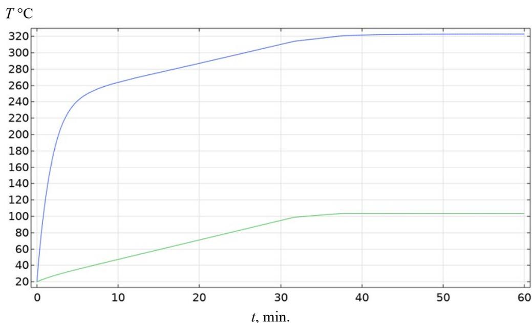
Fig. 6. Temperature dependence on the “hot” (blue curve) and “cold” (green curve) sides of the thermoelectric converter on time.
