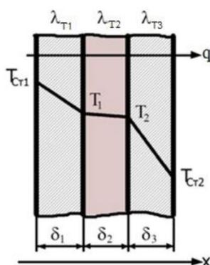
*Fig. 4. Temperature distribution in a multilayer flat wall.*
