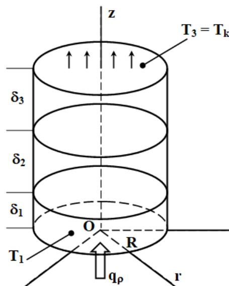
*Fig. 5. Model of a cylindrical three-layer structure.*
