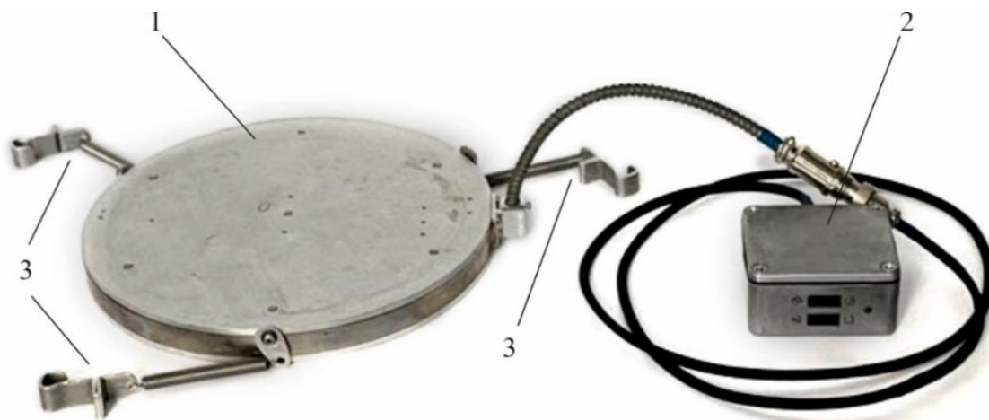
Fig.2. Appearance of universal thermoelectric generator: 1 – thermoelectric generator; 2 – electronic unit of output voltage stabilization; 3 – hooks on springs for attaching the generator to a water tank
