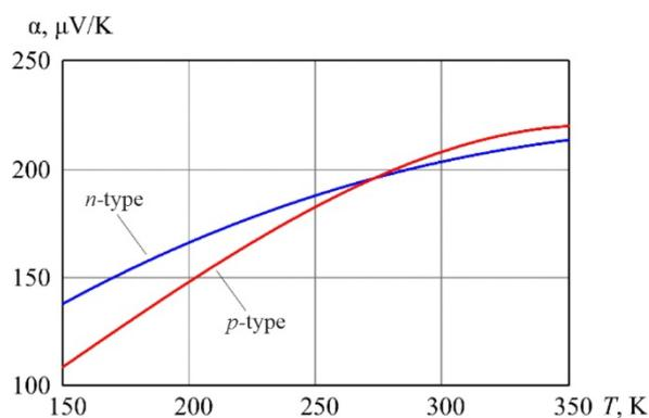
Fig. 2. Temperature dependence of thermoelectric coefficients.
