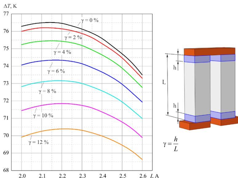
Fig. 6. Dependence of the temperature difference  $\Delta T$  of the thermoelement on the value of the supply current  $I$  and the relative height of the bandage coating  $\gamma = h / L$  ( $h$  – the height of the bandage,  $L$  – the total height of the half-element).
