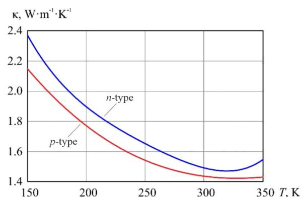
Fig. 4. Temperature dependence of thermal conductivity coefficients.
