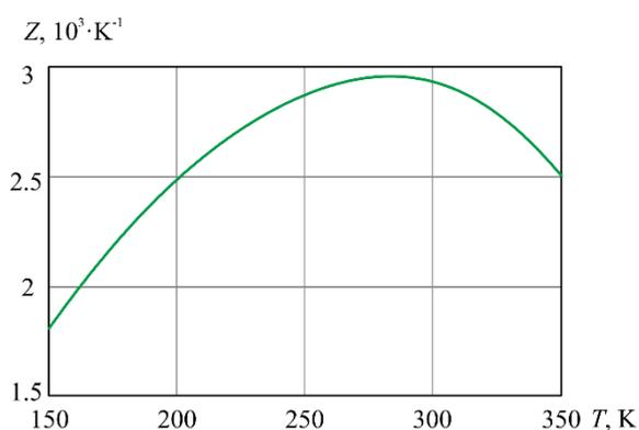
Fig. 5. Temperature dependence of thermoelectric figure of merit.
