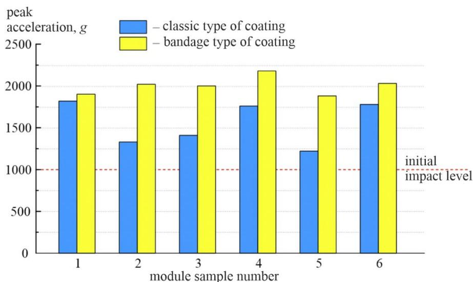
Fig. 7. Impact resistance of thermoelectric modules with anti-diffusion nickel coatings of classic and bandage types.
