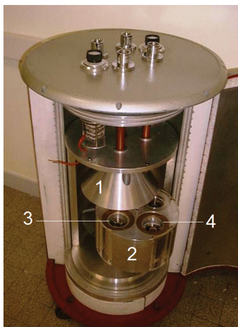
Fig. 4. Microcalorimeter with a Tian-Calvet type heat fluxmeter. 1 – cone of equal temperature distribution, 2 – central cylinder of the thermostat containing thermopiles 3 and 4 (the other two are located behind) with approximately a thousand chromel-alumel junctions each
