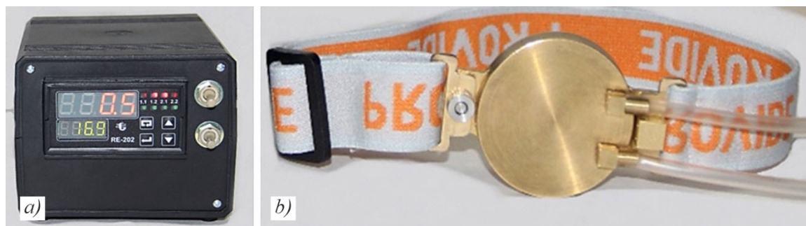
Fig. 6. Appearance of the device for contact cooling of the eye. a). Thermoelectric electronic cooling, control and power unit. b). Coolant heat exchanger
