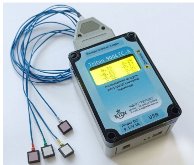
Fig. 1. Thermoelectric device for measuring temperature and heat fluxes
