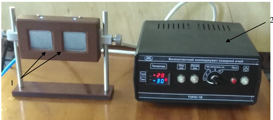
Fig.1. Experimental prototype of thermoelectric device for non-contact cooling of the human eyes: 1 – thermoelectric cooling modules, 2 – electronic control and power supply unit
