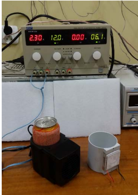
Fig. 1. Car beverage cooler Car mini-cooler \Phi M 201.001 (left), separately to the right - its container with a thermoelectric module installed on it.
