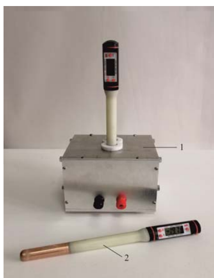
Fig.1. Thermoelectric device for treatment of skin diseases: 1 – thermoelectric cooling unit, 2 – work tool
