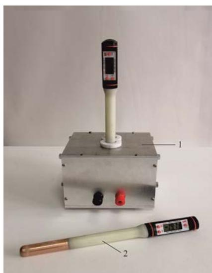
Fig.1. Thermoelectric device for treatment of skin diseases:
