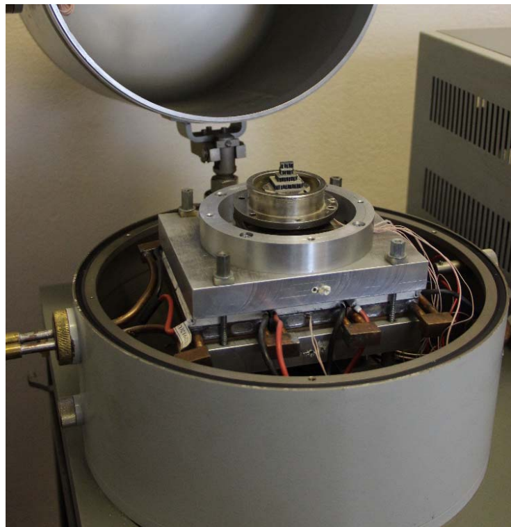
Fig. 2. Appearance of thermoelectric cooling module for an X-ray radiation detector
