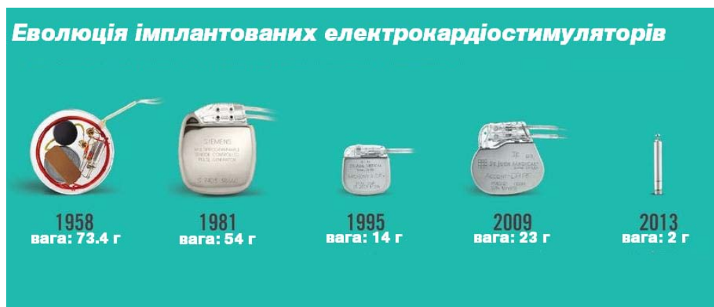
Fig. 9. Evolution of the technology of manufacturing cardiac pacemakers Evolution of implanted cardiac pacemakers. 1958 Weight 74.4 g
