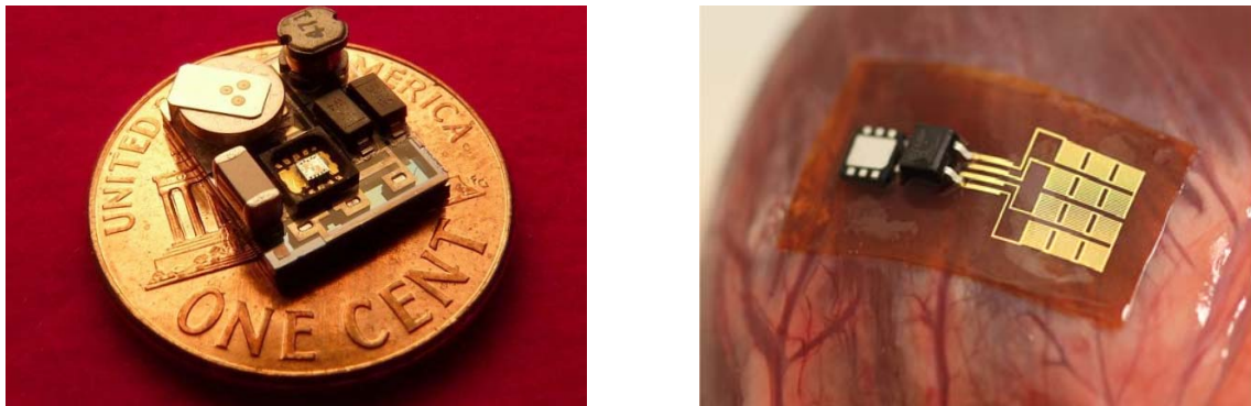
Fig. 13. Piezoelectric generator for cardiac pacemakers [62]
