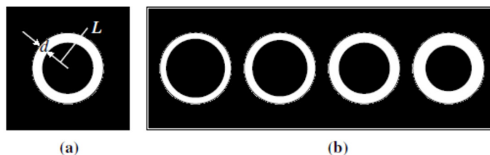
Fig. 7. A separate element of the circular structure (a) and the structure as a whole (b). Black areas – metal [10].
