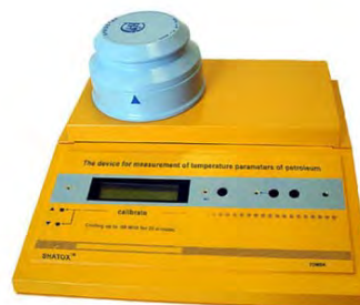
Fig. 4. “CRYSTAL” measuring device for low-temperature indicators of oil products.
