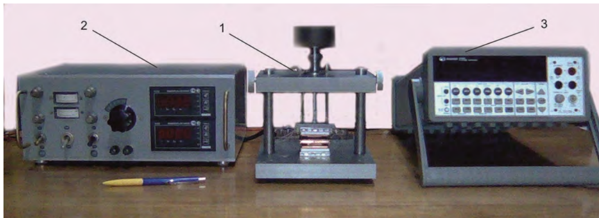
Fig. 1. Visual inspection of the bench for analysis of metrological properties and calibration of thermoelectric heat flux sensors (HFS).
