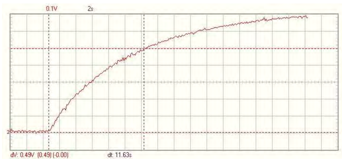
Fig. 5. Time characteristic graph of thermoelectric HFS with dimensions of 16 \times 16 \times 3 mm, equipped with ceramic receiving surface.
