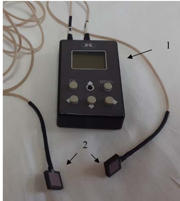
Fig. 1. Thermoelectric device for diagnosing inflammatory processes and pain degenerative-dystrophic diseases of human lumbosacral spine: 1 – control unit, 2 – thermoelectric temperature and heat flux sensor
