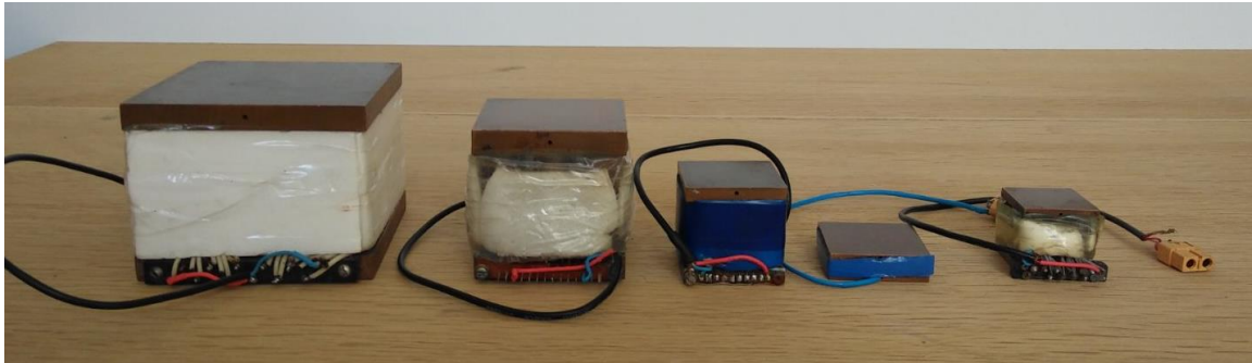
Fig. 3. Heat meters of different sizes for equipment for determining the parameters of thermoelectric generator modules by the absolute method
