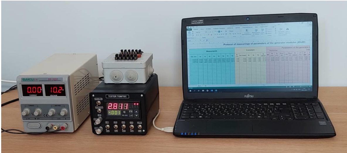
Fig. 4. Appearance of automation system for measuring parameters of thermoelectric modules.
