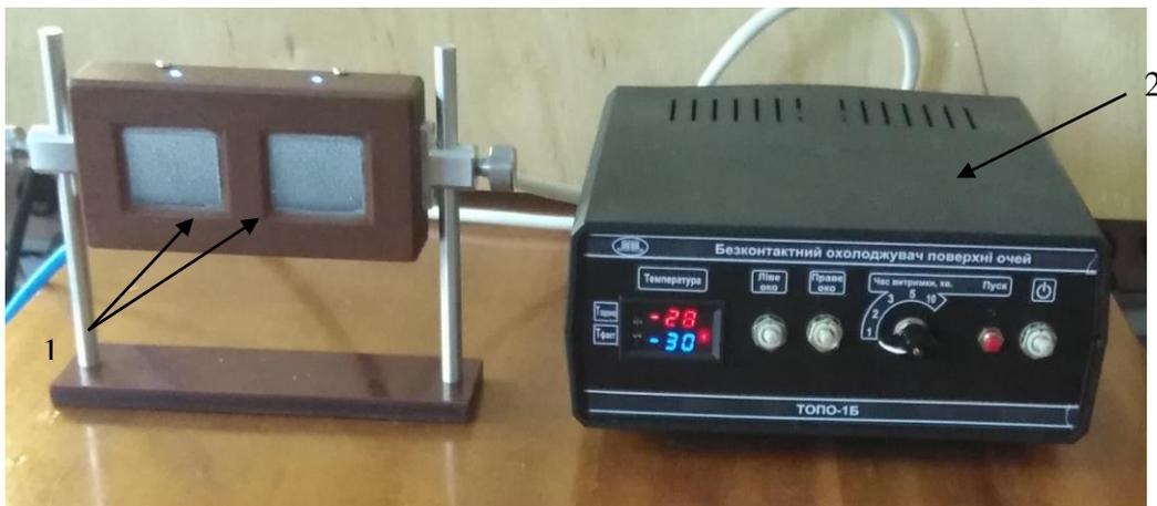
*Fig.1. Experimental prototype of thermoelectric device for non-contact cooling of the human eyes: 1 – thermoelectric cooling modules, 2 – electronic control and power supply unit*
