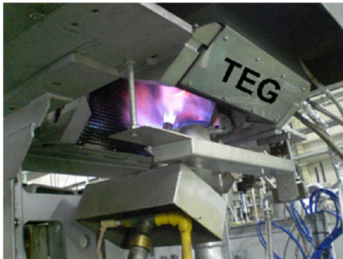
Fig. 4. Installation of thermoelectric generator on cement kiln of the Awazu plant of company Komatsu (Japan) [31].
