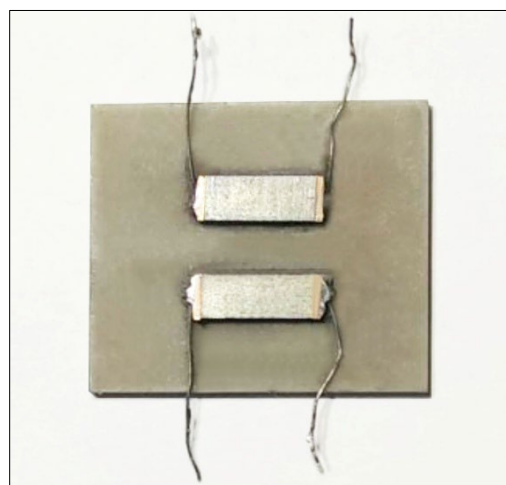
Fig. 7. Beryllium oxide substrate with samples for contact resistance measurement
