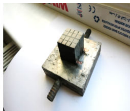
Fig. 4. Photo of a thermoelectric module attached to a water cooler (1×0.4)
