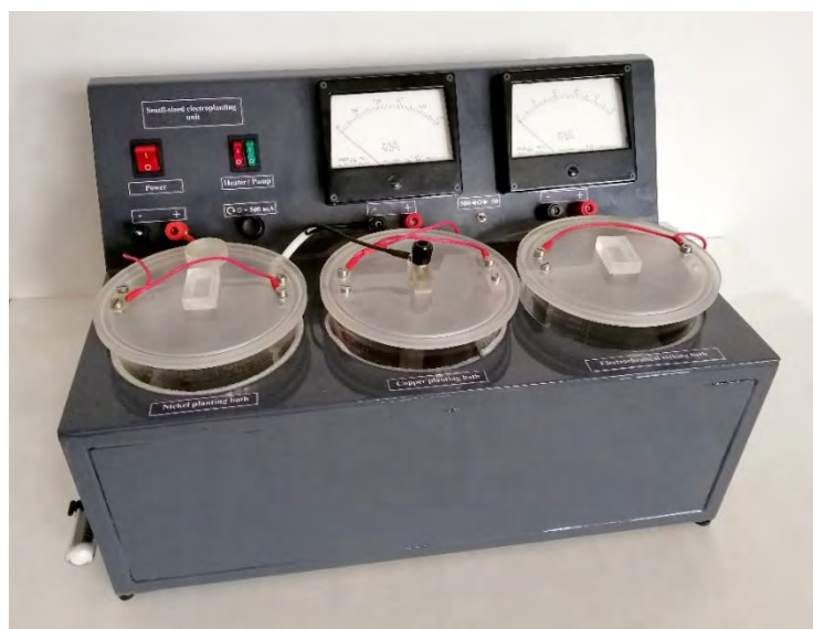
Fig. 10. Appearance of the installation for creating contact structures on measured samples of thermoelectric materials.
